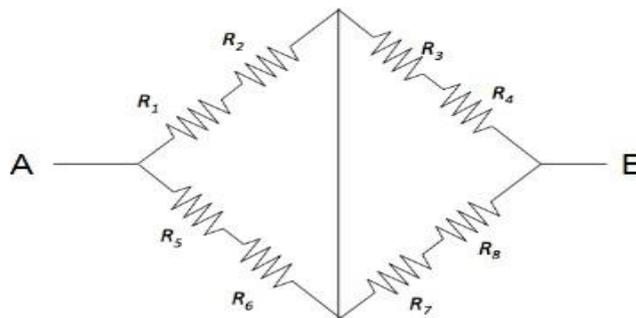
(ii) Find the equivalent resistance for the circuit shown below.
