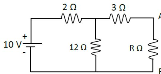
3. (a) Determine the mesh currents for the circuit shown below. [L4][5M]
